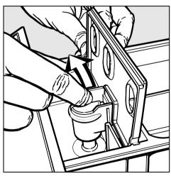
■ Remove the siphon tube from compartment (a) and rinse in warm water.
